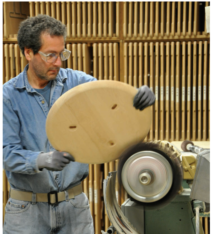
Sanding a seat at Newport Furniture Parts in northern Vermont.
